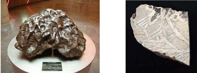
The photo right is an example of the Widmanstätten pattern which is the most commonly found and indicates an average to high nickel content – octahedrites. Hexahedrites have a low nickel content.
